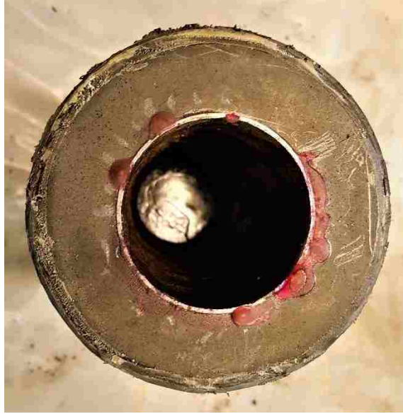
Figure 6. Bottom of a sample after injection, which shows that the epoxy entered the microannulus at the top, flowed through and came out of the bottom.
