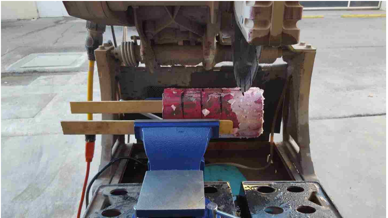
Figure 7. An MK brick saw with vise and wood cushions was the sectioning setup used.
