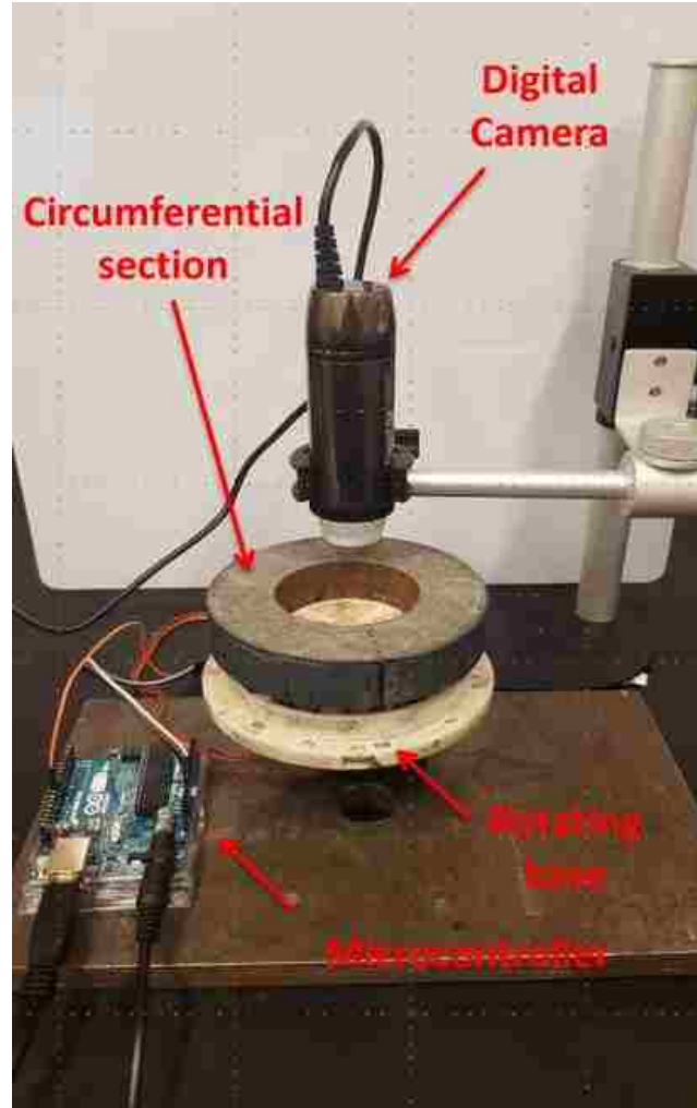
Figure 9. Automated rotating photographic system, comprised by a servo motor controlled by an Arduino board and a servo motor.
