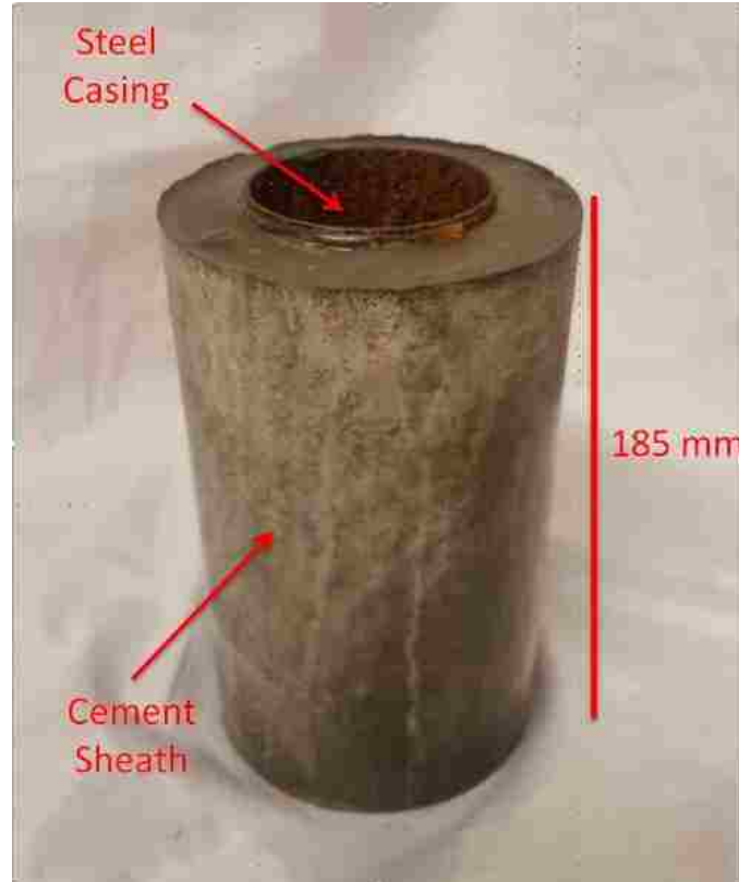
Figure 1. Finished wellbore-shape specimen, comprised of a steel casing and a cement sheath.
