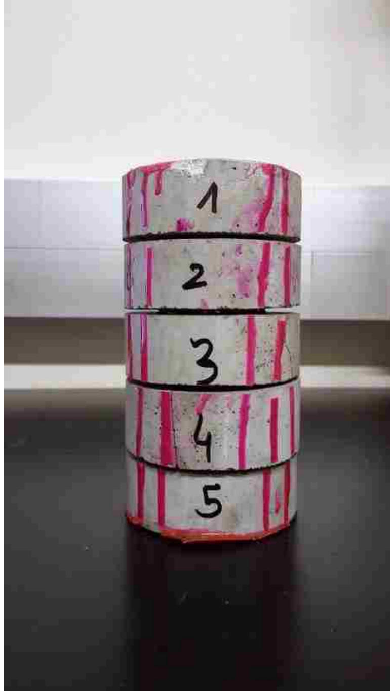
Figure 8. Wellbore specimen A sectioned, with all the circumferential sections labeled.
