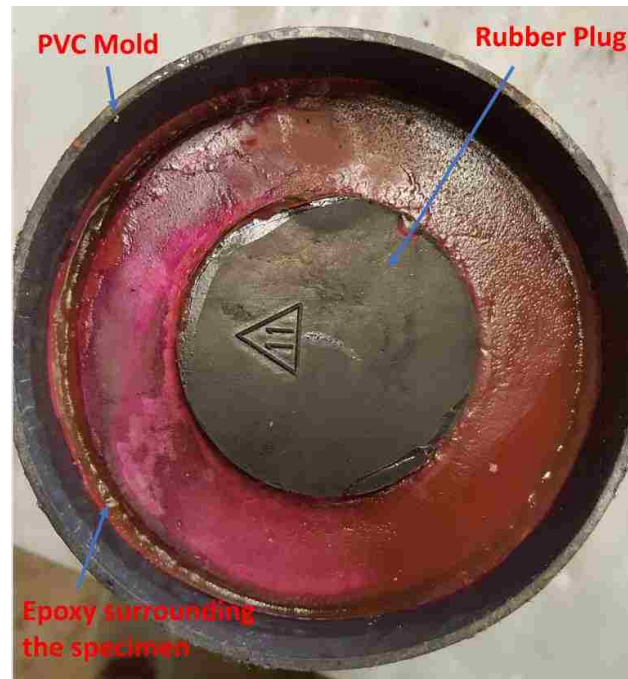
Figure 4. Wellbore specimen inside the PVC mold with the surrounding epoxy and the rubber plug, ready to pour the epoxy over it and place the specimen in the injection system.
